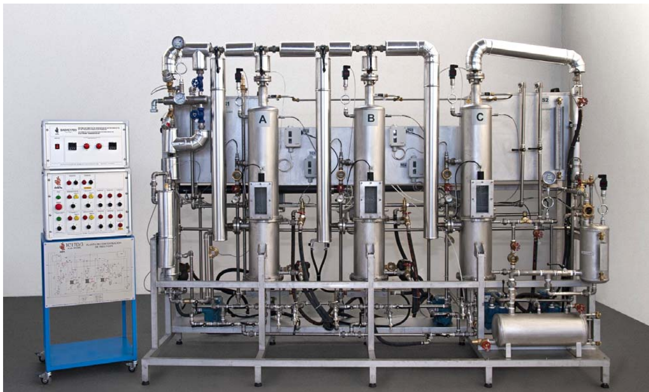
IC17D/3 –Triple Effect Concentrator (Code 991000) with optional SAD/IC17D3 Automatic Data Acquisition System
