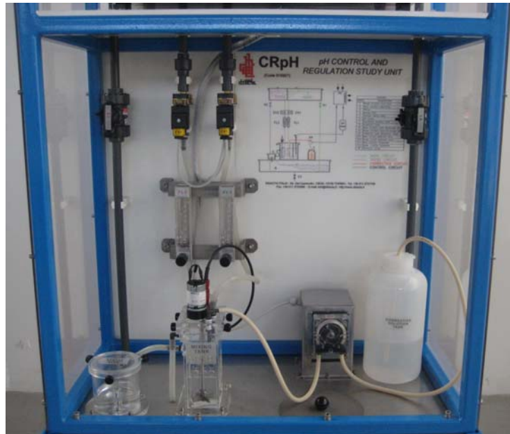
Figure 1 – Process Control Equipment
